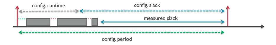
$$perf\_index = \frac{measured\_slack}{config\_slack}$$
