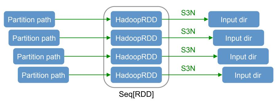
Sequentially listing input dirs via S3N file system.
