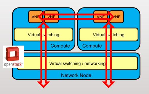
VNF (North-South) and service chain (East-West) throughput is limited by Linux virtual switching / networking capacity
