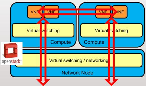
VNF (North-South) and service chain (East-West) throughput is limited by Linux virtual switching / networking capacity
